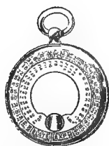
B. Watkins' Watch-form Exposure Meter
