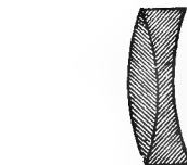
D. Simplest Form of Single Achromatic Lens
